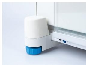
Fully automatic balance levelling
