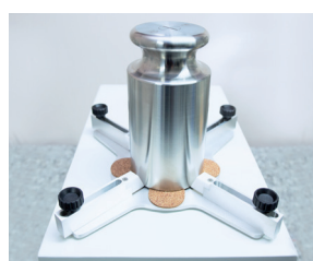
Weighing pan with mechanical system for weights positioning
